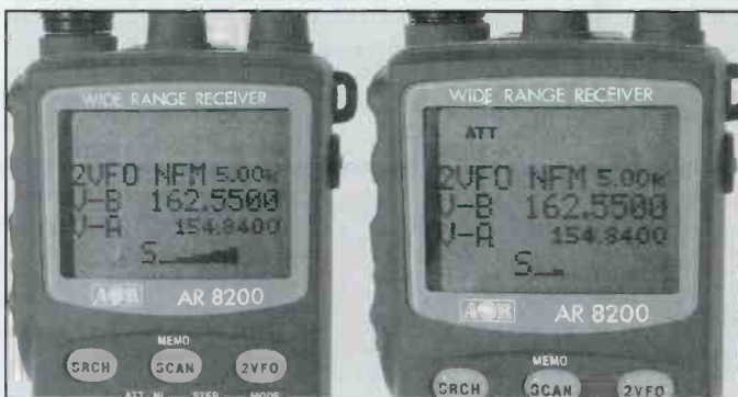
Here's a before and after comparison. Note the S-meter and the drastic drop in signal after the attenuator is turned on. That's how they work!
