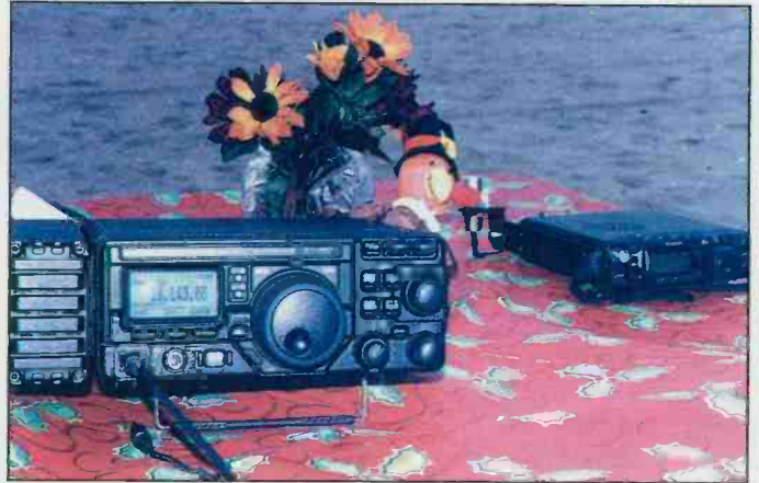
The box on the side of the FT-897 is the optional antenna tuner.
