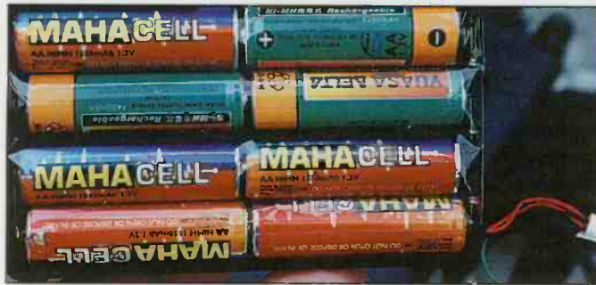
These long life MAHA supercells play twice as long as NiCads! Cut the FT-817 green wire to charge.
