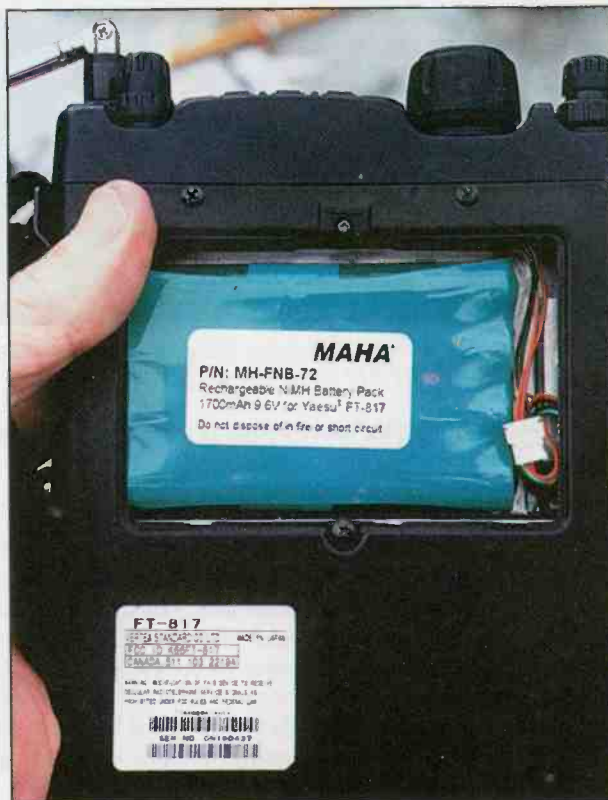
The MAHA NiMH 1700 mAh pack inside the FT-817 – just plug it in.
