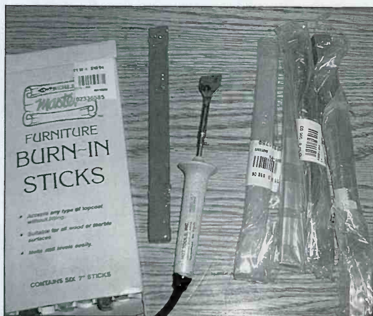
Photo 2: Some of the basic materials needed for lacquer stick repairs. The lacquer knife, and an assortment of various lacquer sticks which were chosen to match the walnut and other common finishes encountered on vintage radios.
